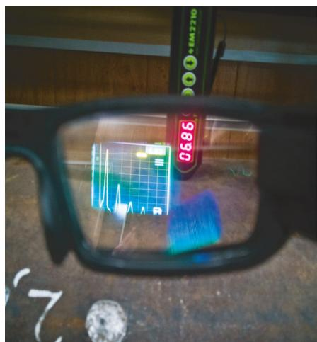
EM2210 mini thickness gauge can be supplemented with **AR glasses** upon your request. AR glasses allow using the EM2210 in hard-to-reach places, where display readouts are impossible or difficult. In this case the readouts are displayed on the lenses of AR glasses and the operator can always see them.
