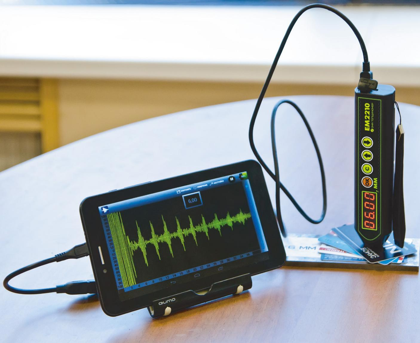
**EM2210 is easily calibrated** using specified thickness or sound velocity.
